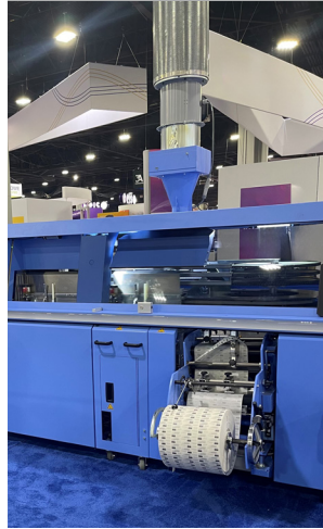
Muller Martini Vareo running LBS endsheets and reinforcing materials
