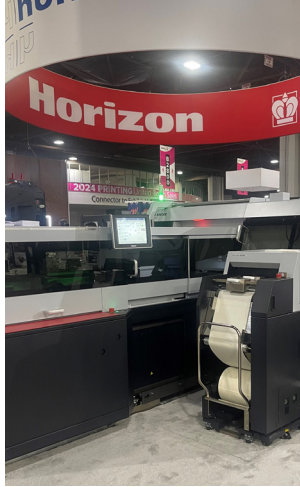
Standard Horizon BQ-500 running LBS endsheets and reinforcing materials
